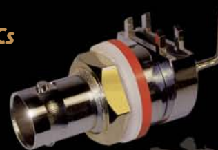
GRBNC R Right angle, PC board mount BNC. Non magnetic, eutectic Brass, Rhodium plate. Thin Brass nut, Gold plate.
