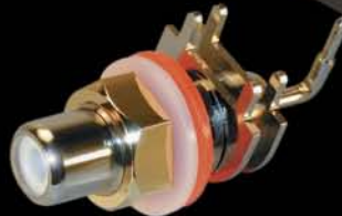
GRFA P RT2 Thick Two piece, right angle, PC board mount female RCA. Non magnetic, eutectic Brass, Rhodium plate. Thick Brass nut, Gold plate.
