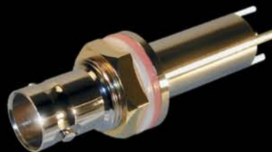
GRBNC S Straight, PC board mount BNC. Non magnetic, eutectic Brass, Rhodium plate. Thin Brass nut, Gold plate.
